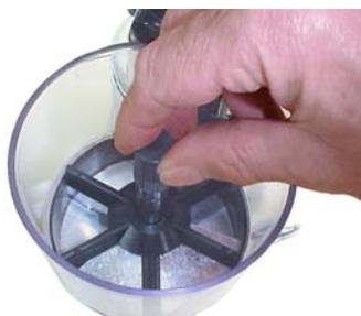
While making this adjustment, place a finger or thumb into the dispensing unit outlet so the wheel is prevented from turning.
