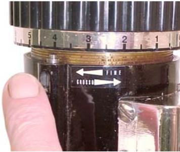
The grinding adjustment wheel will move freely while the locking pin is held down. It's important to move the grinding adjustment wheel **only one notch at a time**, then to release the locking pin. A small change in the grind texture can make a big change to the flow of coffee.
