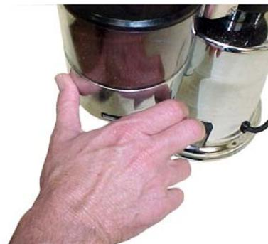
It's important when adjusting the dosing quantity to *roll the coffee*. This is done by placing the dispenser lid under the dosing unit outlet and operating the dosing lever so coffee grounds fall onto the lid. Do this about five times then return the ground coffee on the lid back into the dispensing unit. Repeat this process once more to ensure all six dosing chambers have been evenly filled.
